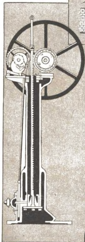
Right—Watt's double acting steam pumping engine. Below—an early form of Otto and Langen's single cylinder gas engine.
